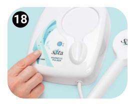
If at any time during your session you want to turn the unit OFF, press and hold the ON/OFF/MODE button for 2 seconds.
