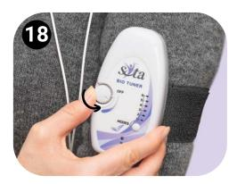
To turn the unit OFF rotate the ON/OFF switch counter clockwise until it clicks.
