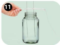
Put the Silver Wires back into the solution and use them to stir the solution for a few seconds.
