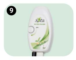
The GREEN light will be ON and the ORANGE light will come ON showing that the Silver Wires have conductivity and are making the lonic~Colloidal Silver.
