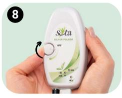
Turn the unit ON. No need to adjust the intensity level as that is only for micropulsing.
