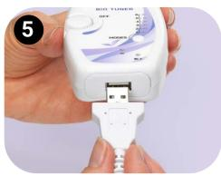
Plug the Bio Tuner Cord into the unit.
