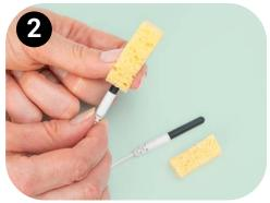
Slip the Sponge Sleeves over the Rubber Probes. You may need to gently twist to slide the Sleeves over the Probes.
