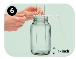
Keep the wires 1-inch from the bottom of the container.
