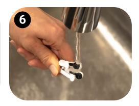
Moisten the Rubber Electrodes in the Ear Clips with some water.
