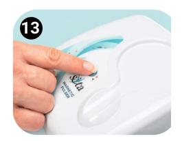
Touch the SOUND ON/OFF button once more (twice) to hear a BEEP each time the magnetic pulse is released.
